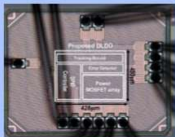
Chip micrograph of the proposed Digital Low-Dropout Regulator, W. Tsou et al., ISSCC 2017
